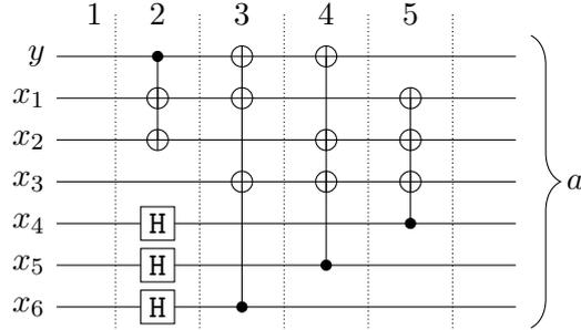
Figure 2: Encoding circuit for the Steane  $[[7, 1, 3]]$  code
